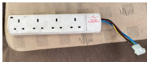
Old PDU connector fitted to mains extension
